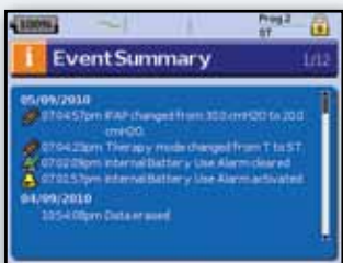
The Event Summary screen provides a quick overview of the main events, such as setting changes and alarms
