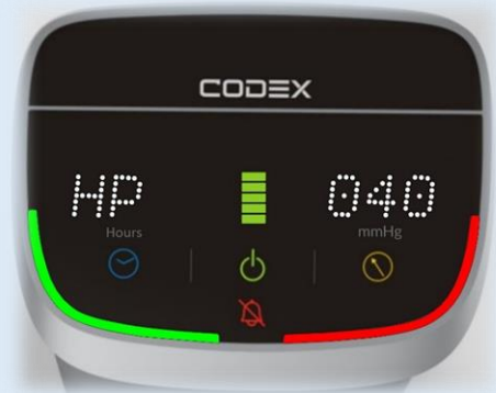
Both sleeves connected, HP Alarm for the right sleeve
