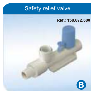
When an occlusion occurs in the inspiratory branch, the circuit relief valve will limit the pressure excess in the line, designed to operate with a pressure of 17cmH 2 O at flow of 8L/min
